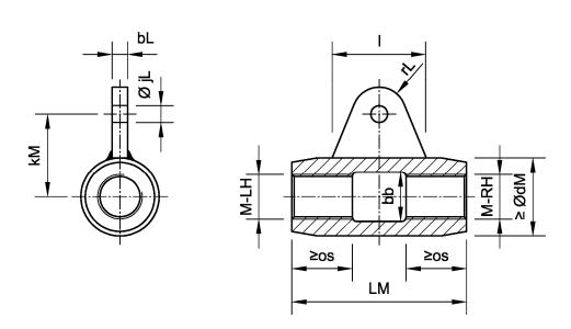
Minimum screw-in length of the tension rod = om - oj according to Annex B3
